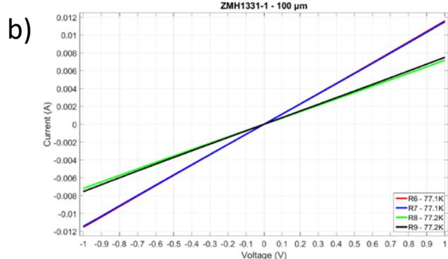
Fig. 1: a) Typical ZnO MESA RTD structures after fabrication. B) Exemplary IV-curve of a  $100\mu\text{m}$  square MESA RTD structure at liquid nitrogen temperatures.
