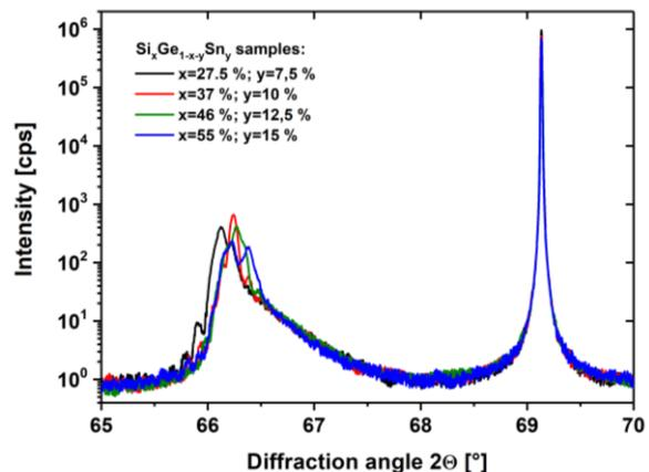
Fig. 1: XRD pattern of  $\text{Si}_x\text{Ge}_{1-x-y}\text{Sn}_y$  layers with different composition
