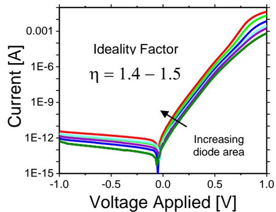
Fig. 1: I-V Characteristics for different sized diodes
