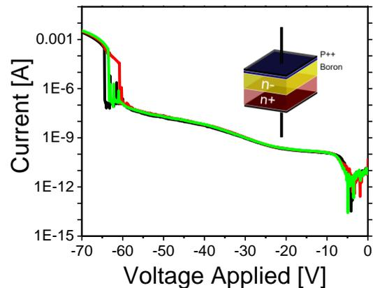
Fig. 2: Reverse Breakdown Characteristics
