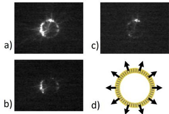
Fig.1: (a) Unpolarized nearfield measured with a bolometer camera. (b) Vertical orientation of the wire grid. (c) Horizontal orientation and (d) resulting polarization of the electric field.
