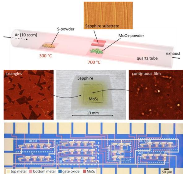
Fig. 1: Schematic of the CVD tube furnace with AFM image of the bare sapphire substrate and the optical microscope images of the grown films on the wafer. On the edge of the grown film triangular shape grains are formed, which then coalesce into continuous film towards the center of the wafer. On the bottom, optical microscope image shows 1-bit microprocessor, consisting of 115 transistors.
