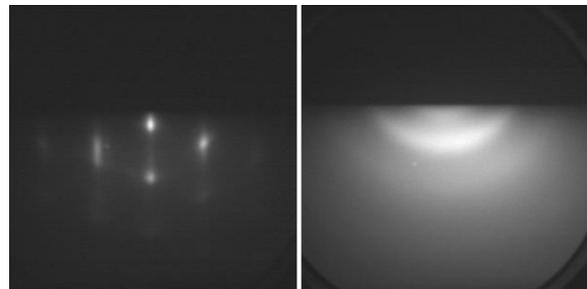
Fig. 1: RHEED images show the surface structure of a (111)Si substrate when exposed to oxygen only (left), and when silicon and oxygen are deposited simultaneously (right). The duration of both experiments was 30 min.
