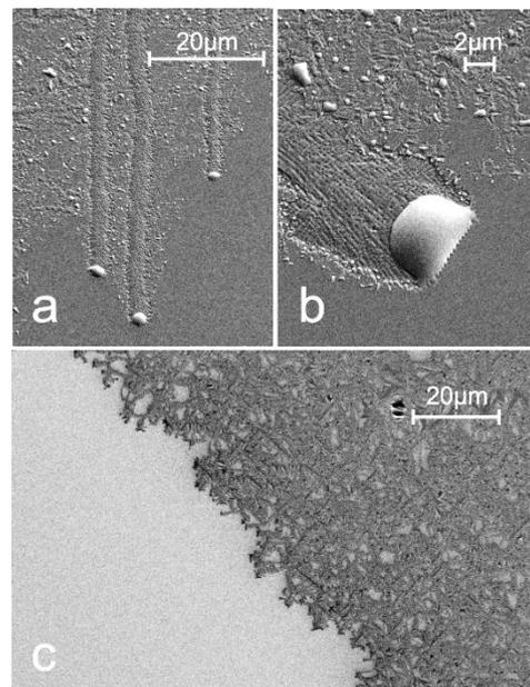
Fig. 1: SEM images taken from real-time video sequences of the precipitate-induced phase separation process in GeSn epilayers. The Sn droplets in (a) and (b) appear bright, the corrugate trails consist of single-crystalline Ge. (a) and (b) were recorded in-vivo at  $250^\circ\text{C}$ , (c) at  $350^\circ\text{C}$ .
