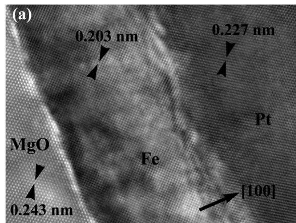
Fig. 1: High resolution transmission electron microscopy image from an epitaxial grown Fe/Pt bilayer. The {111} MgO, {011}Fe, and {111}Pt lattice fringes are clearly resolved, along the [011]MgO-Pt//[001] Fe projection direction [4].
