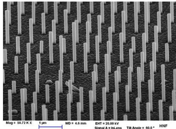
Fig.1: SEM image of an InAs/GaSb core-shell NW array.
