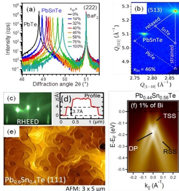
Fig. 1: (a) XRD pattern, (b) reciprocal space map around the asymmetric (513) reflection, (c) RHEED pattern, (e) AFM image with (d) line profile and (f) ARPES spectrum for (111)  $\text{Pb}_{1-x}\text{Sn}_x\text{Te}$  epilayer with  $x_{\text{Sn}}=0.46$ .
