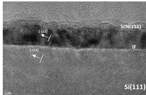
Figure 1: HRTEM image of ScN 8nm thick. The normal directions to the (-111) planes are indicated by white arrows.
