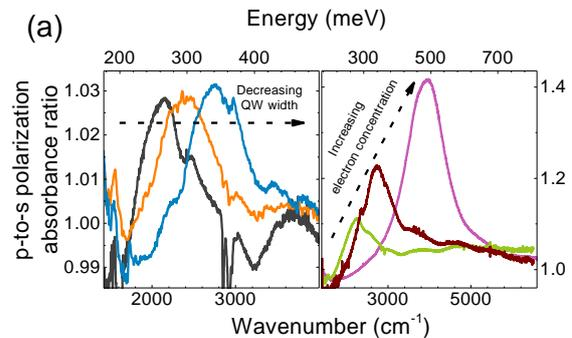
Fig. 1: p to s polarization absorbance ratio for the MQW structures presented here for (a) different QW widths (b) different n-type doping.
