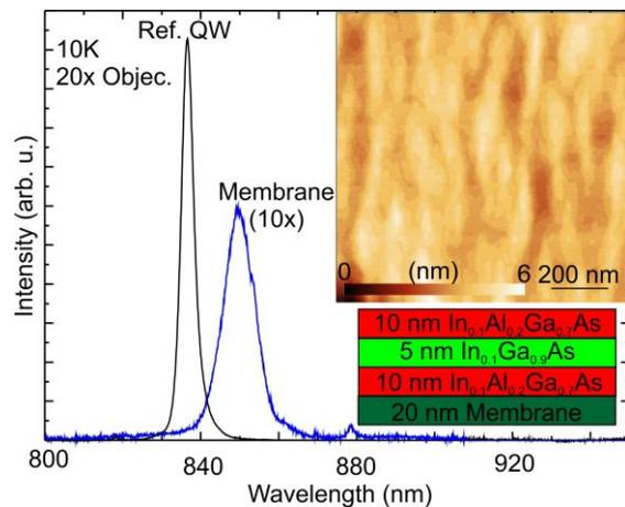
Fig. 1: Photoluminescence spectrum obtained from an InAlGaAs/InGaAs/InAlGaAs quantum well grown on a released and relaxed membrane or a GaAs (001) substrate as reference. The upper inset shows the AFM topography of the quantum well on the membrane, the lower the grown structure.
