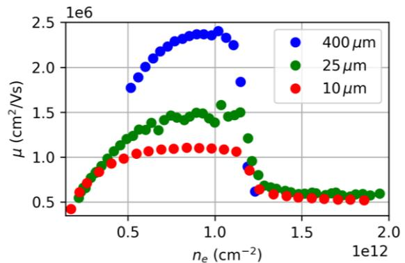
Fig. 1: Measured electron mobilities at 1.3 K of an InAs QW with varying Hall bar widths.
