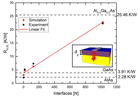
Fig. 1: The thermal resistance of a superlattice increases linearly with number of the interfaces. Reference values of bulk film are plotted as dashed lines. Inset: Thermal waves, excited by an oscillating current in the heater stripe, penetrate into the epitaxial superlattice to determine the influence of interfaces on the thermal conductance.
